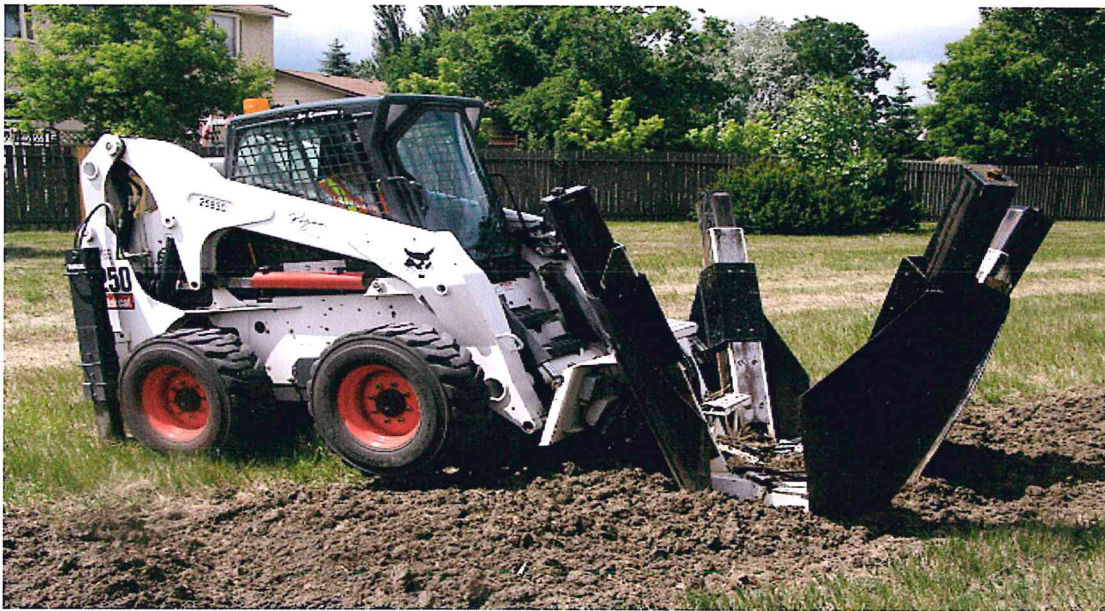
Tree spade unit - excavating a deep enough hole to plant trees in the SE section of the city.
